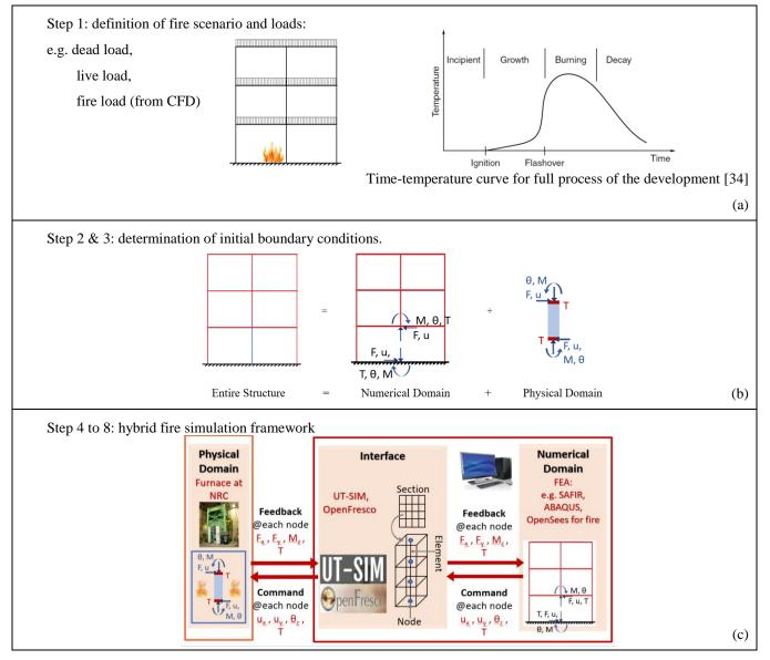
Figure 5. Process of hybrid fire simulation.
